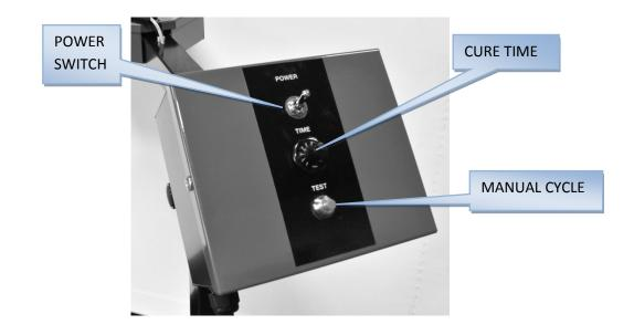
POWER SWITCH - ON/OFF POWER 120 VAC 20 AMP CURE TIME – TIME FOR QUARTZ BULBS TO STAY ON MANUAL CYCLE – PUSH TO MANUAL ACTIVATE QUARTZ BULBS PHOTO SENSOR:
