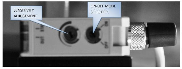
SENSOR MODE OFF = LARGE PALLETS (PALLET STOPS UNDER SENSOR)
