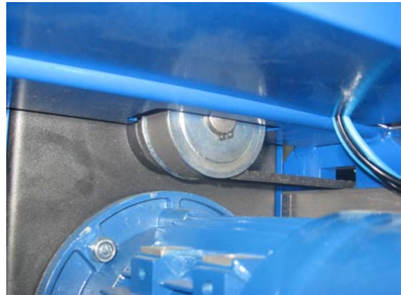
Fig. 27: HEAD DRIVE BELT
